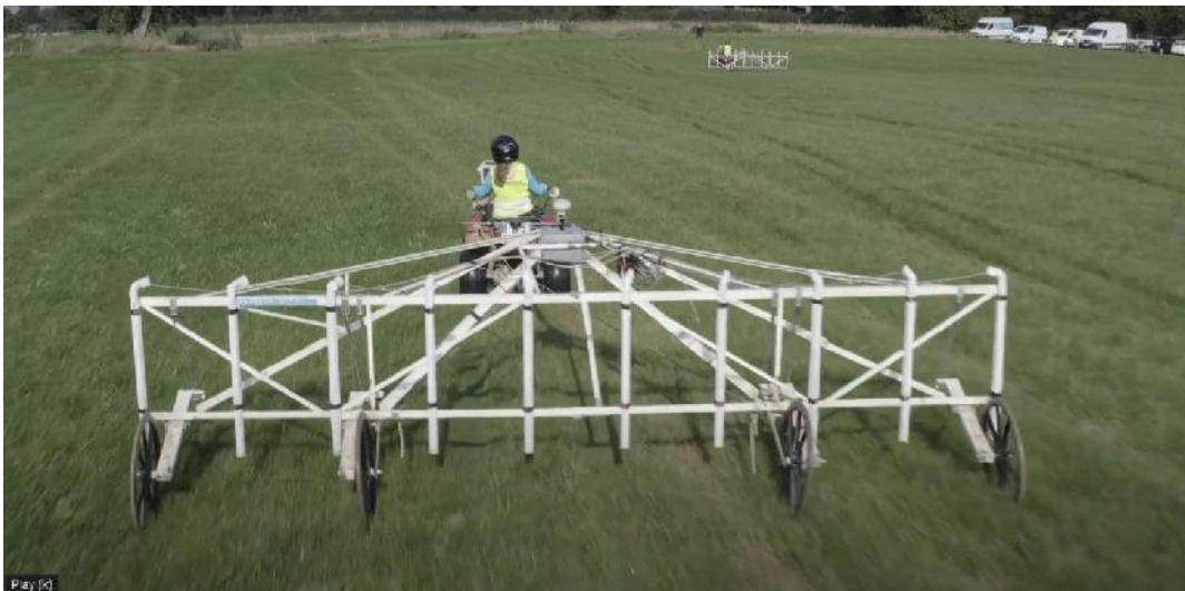
Photo 2: Magnetic Gradiometer with 10 sensors back view
