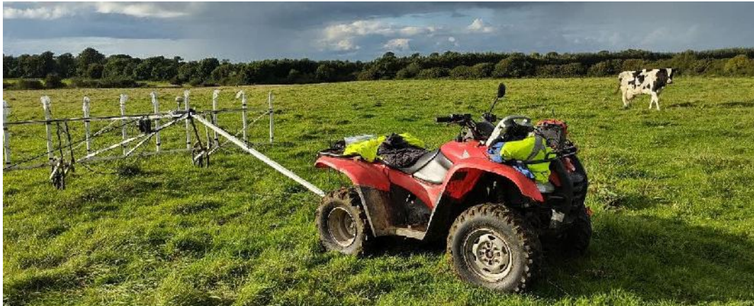
Photo 1: Magnetic Gradiometer with 10 sensors front view
